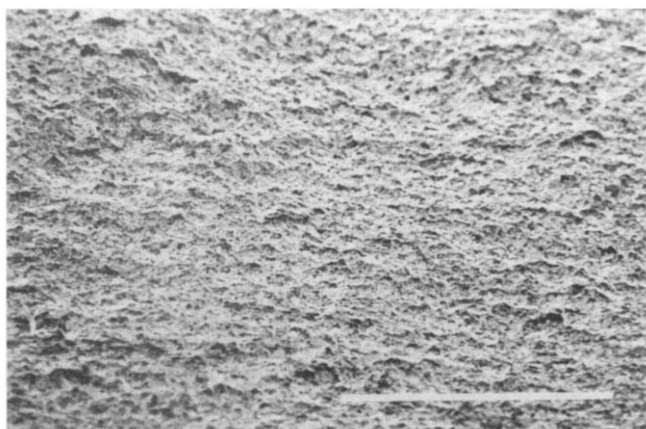
Figure 12 SEM micrograph of the fracture surface of the 70/30 simultaneous full-IPN specimen impact tested at -10°C. Scale bar = 100 μm
